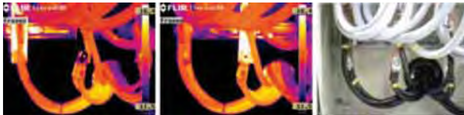
The fact that the 'hot spot' in the middle picture disappears when the location of the thermal imaging camera is slightly altered clearly shows that this apparent 'hot spot' is caused by reflection. This is another tell-tale sign.
