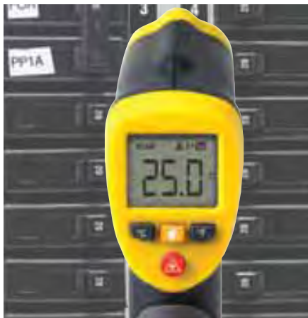
IR thermometer, temperature measurement in one spot
