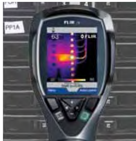
FLIR i3, temperature in 3,600 spots
