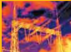
Inspection of high voltage power lines
